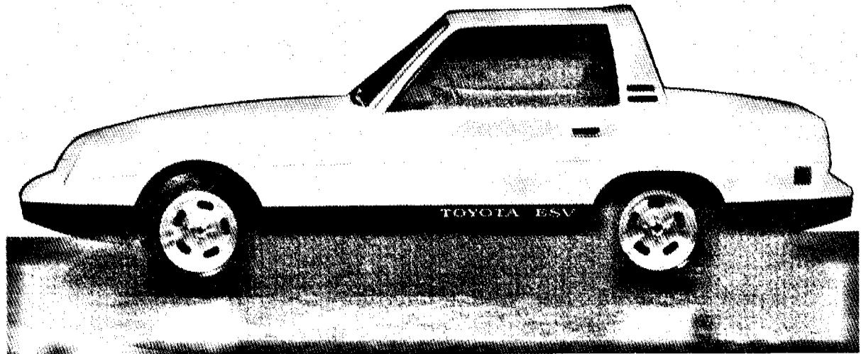
Toyota Motor Company's experimental safety vehicle features an impact absorbing frame and fire wall, an engine that falls away from the vehicle upon impact, self-inflating protective cushions, reinforced side and roof, automatic skid control, and increased visibility for occupants.
