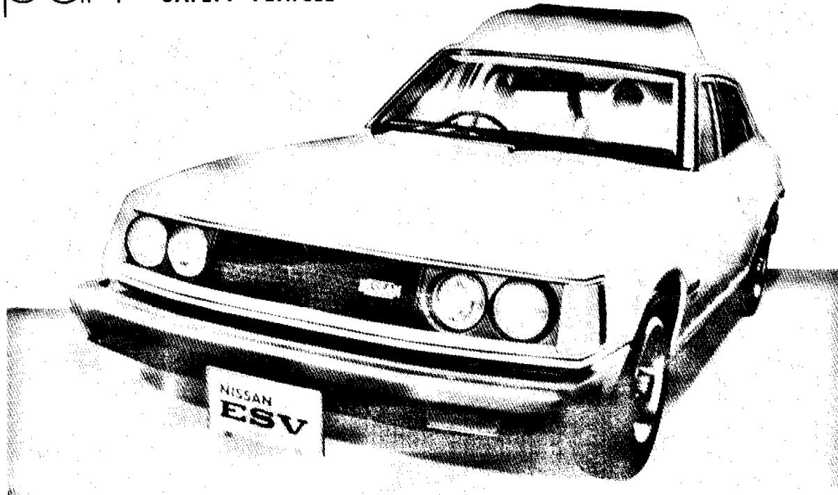
The Nissan Motor Company's ESV is a modified production model of the Datsun 510 sedan designed to insure the occupant's safety in a 50 mph barrier crash.
