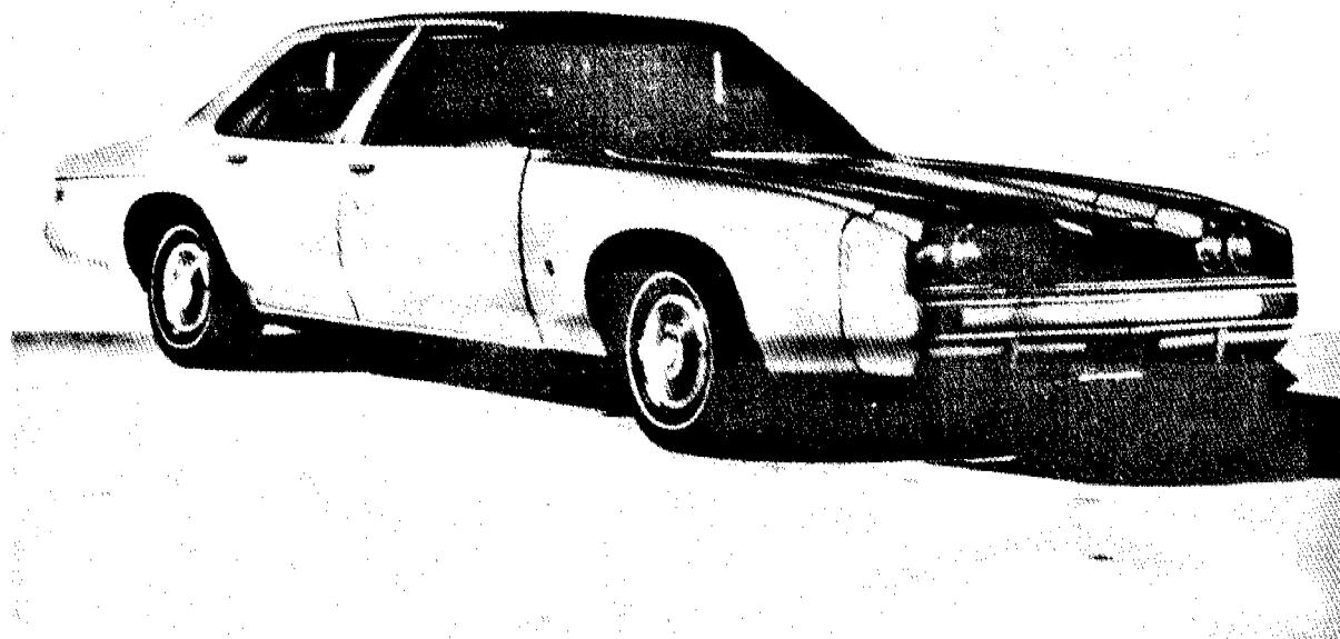
General Motors' ESV prototype uses a specially engineered bumper and energy absorbing frame to afford maximum occupant protection.
