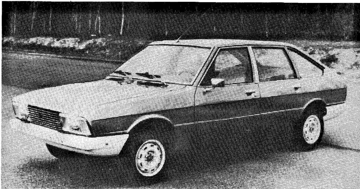
Valiant). Design features of the car include transverse front engine, front drive propulsion system, four-cylinder engine, unitized construction, and five-door (hatchback) layout. All of these features are expected to become increasingly popular in future American family cars.
