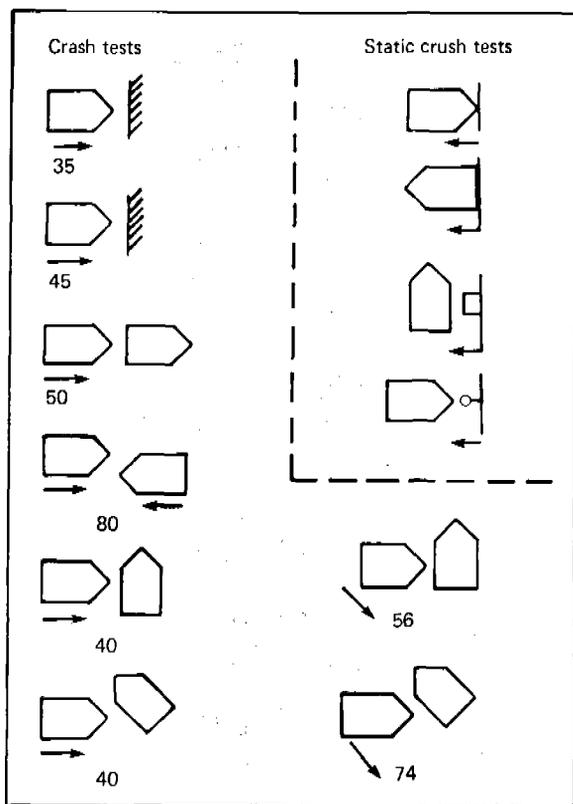
Figure 6. Base vehicle tests (mi/h).
