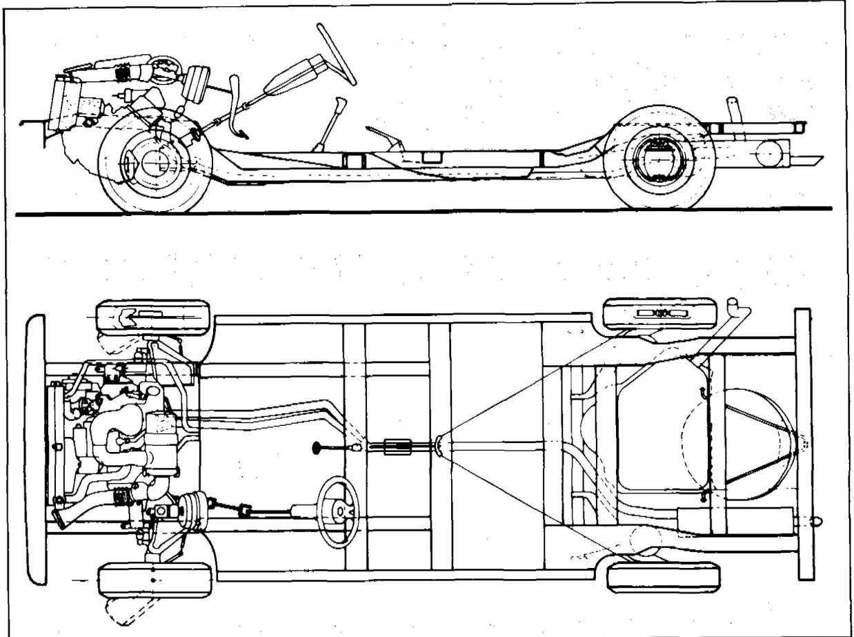
Figure 5. Schematic illustration of the Simca running gear components.
